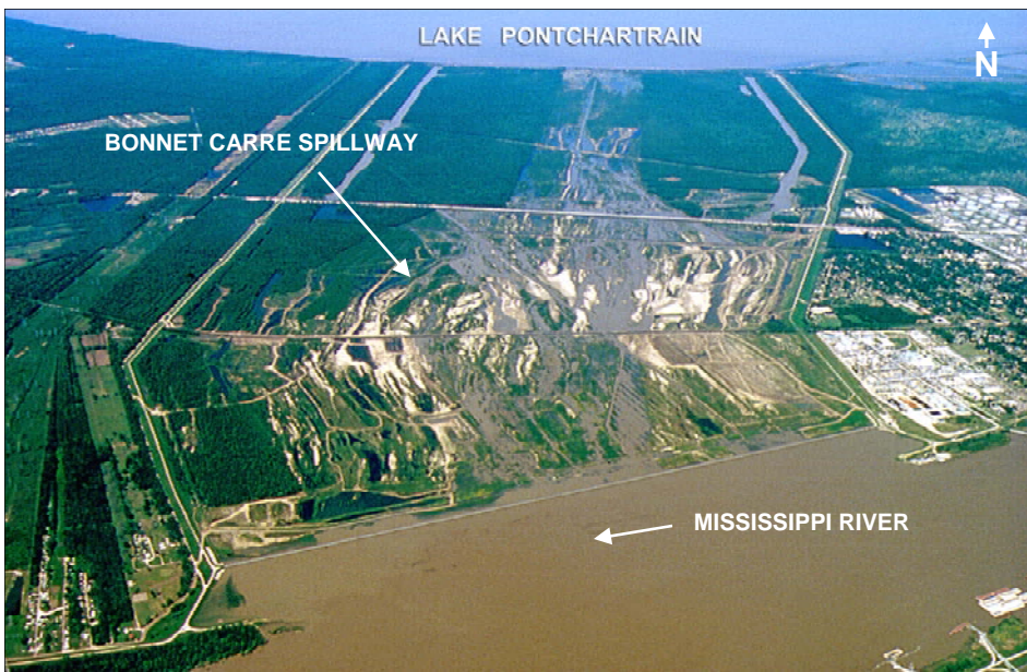
The Bonnet Carré Spillway is 28 miles above New Orleans in St. Charles Parish. It requires about 36 hours to lift the 7,000 wooden needles from its 350 bays. The structure diverts high river water into Lake Pontchartrain.
