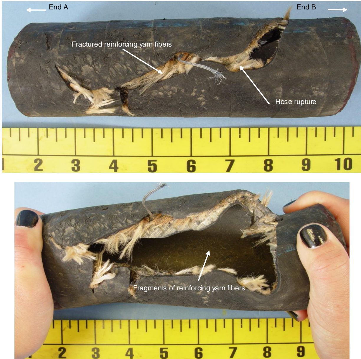
Figure 3. Views of outside (top) and inside (bottom) of ruptured section of accident hose.
