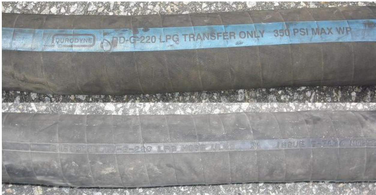
Figure 1. Blue Mylar and imprinted stripes on accident hose.
