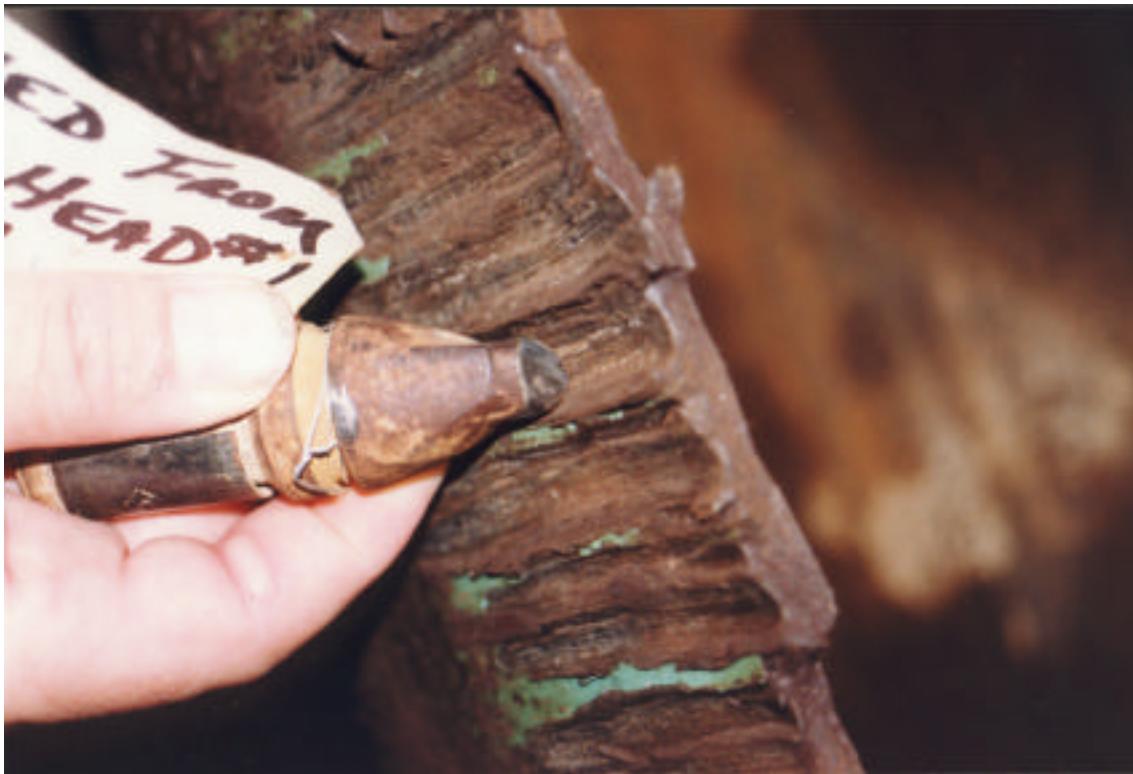
Figure 2. Comparison of cutting tool tooth with gouges found at rupture site
