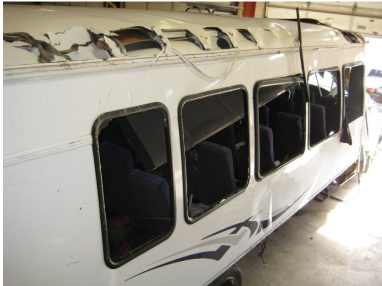
Figure 11. Right side of accident bus roof.
