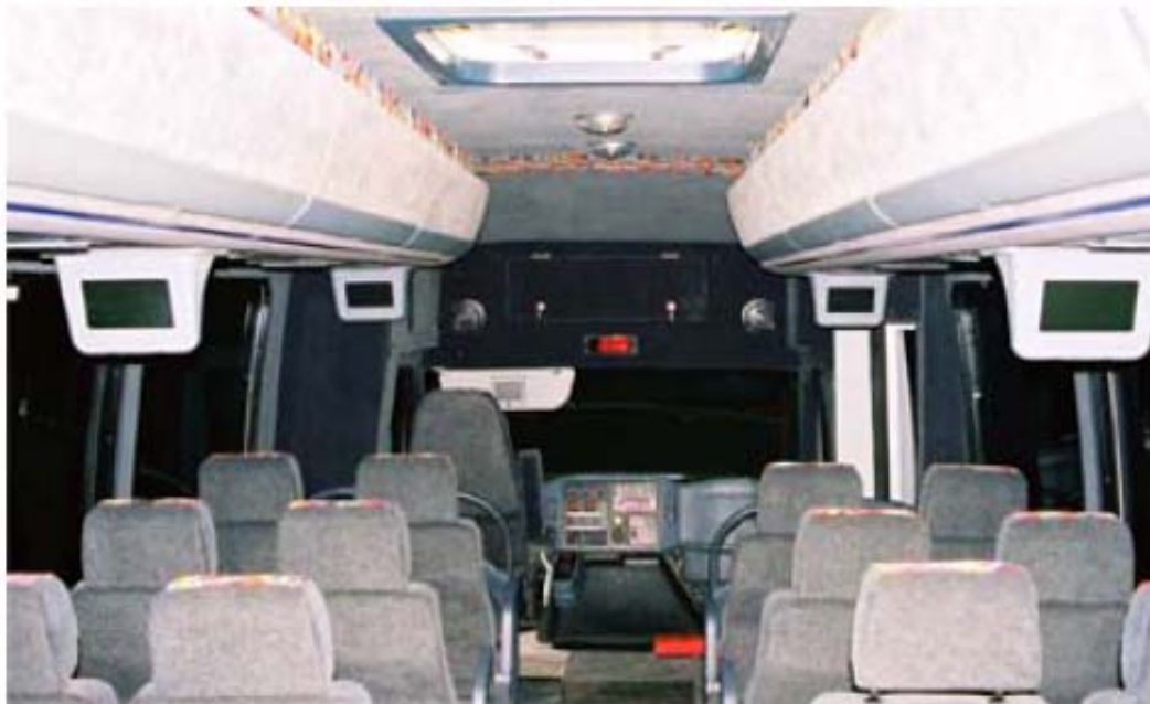
Figure 13. Interior photograph showing seatbacks, televisions, and overhead luggage racks on exemplar Starcraft XLT bus. Note: The accident bus did not have video displays or luggage rack doors.
