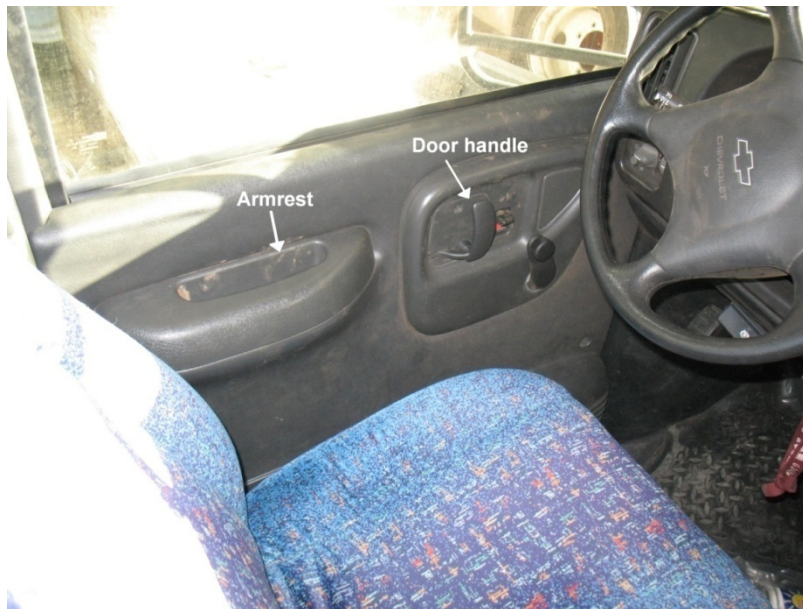
Figure 7. Layout of driver's side door, showing armrest located near seatback and interior door release handle adjacent, to the right.
