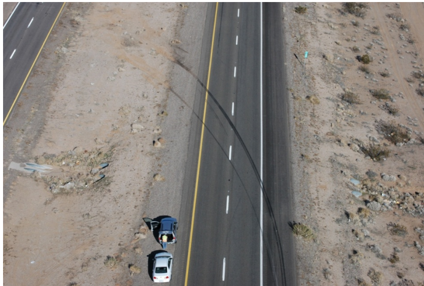
Figure 8. Aerial view of two northbound lanes of US 93, showing tire marks extending from right shoulder, across highway, and onto earthen median.
