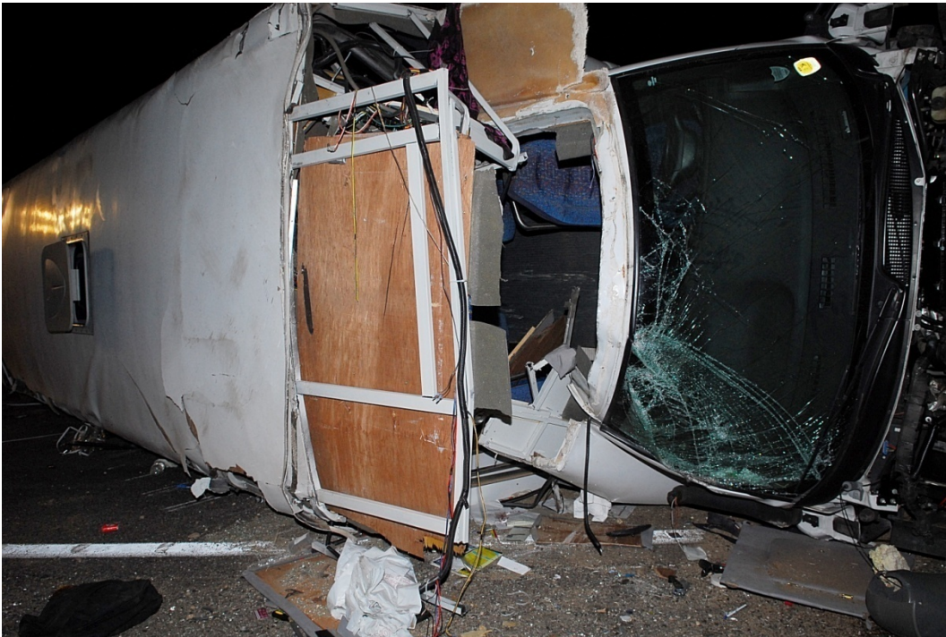
Figure 5. Bus at final rest, on its right side, showing damage to fiberglass front fascia above driver's compartment.
