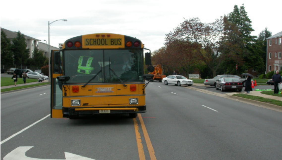
Figure 9. View from the front of an exemplar school bus positioned as the accident bus is likely to have been immediately preceding the accident. Note that the bus's left-front corner is encroaching upon the eastbound lane. (Photograph taken during postaccident reconstruction.)
