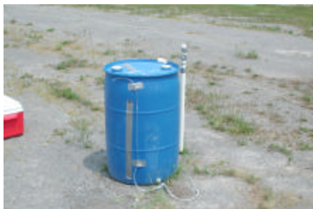
To test for microbial activity, site groundwater is mixed with tracers and nutrients in drums and injected into monitoring wells
