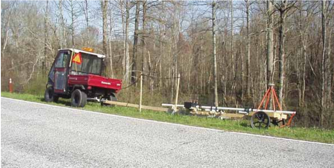
Figure 9. Photo. EM31-3 and ATV on Natchez Trace Parkway.
