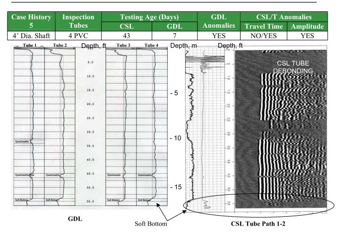
GDL test was performed first which indicated three zones of density anomalies. CSL was performed next with severe PVC tube debonding observed in the 43-days old shaft.
