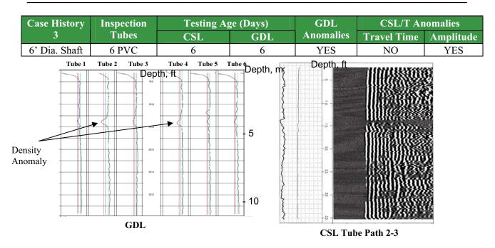
Analysis: CSL and GDL performed at the same time. GDL indicates a density a 4.1-4.4 m (13.5-14.5 ft). CSL indicates low amplitude (reduced signal energy) at the same depth; but no velocity anomaly.
