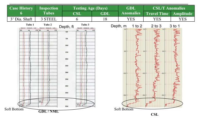
Comprehensive geophysical logging program was performed including: crosshole sonic logging (CSL), 3-D zero-offset tomography (CSLT), gamma-gamma density (GDL), and neutron-moisture logging (NML).
