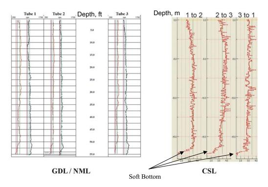
Comprehensive geophysical logging program was performed including: crosshole sonic logging (CSL), 3-D <u>zero-offset</u> tomography (CSLT), gamma-gamma density (GDL), and neutron-moisture logging (NML).
