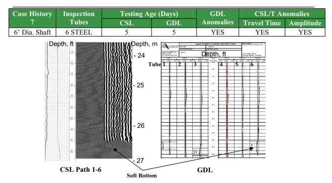
Comprehensive Geophysical logging including: crosshole sonic logging (CSL), 3-D multi-offset tomography (CSLT), and gamma-gamma density logging (GDL) was performed from **steel** pipes.
