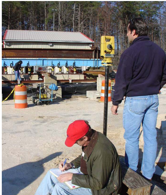
Figure 55. Photo. Total station surveying of footing deflection.
