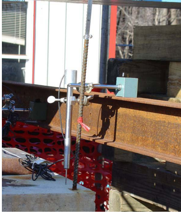
Figure 56. Photo. LVDT instrumentation installation.
