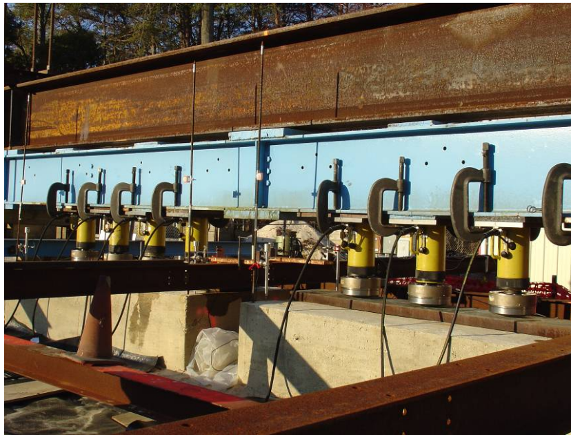
Figure 60. Photo. Field-scale test wall load frame and jack set-up.
