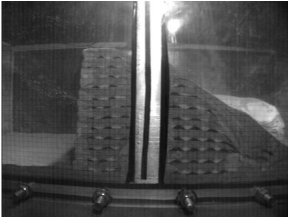
Figure 39. Photo. Centrifuge test series 2 at 38g acceleration.
