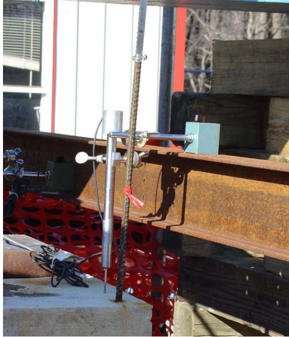
Figure 56. Photo. LVDT instrumentation installation.
