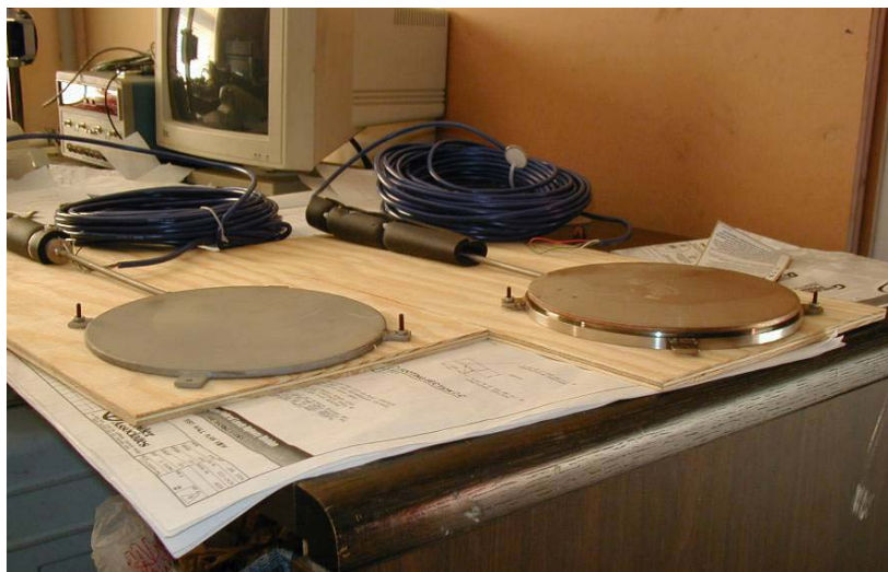
Figure 53. Photo. Earth pressure cells, Model 4800 (left) and Model 4810 (right).
