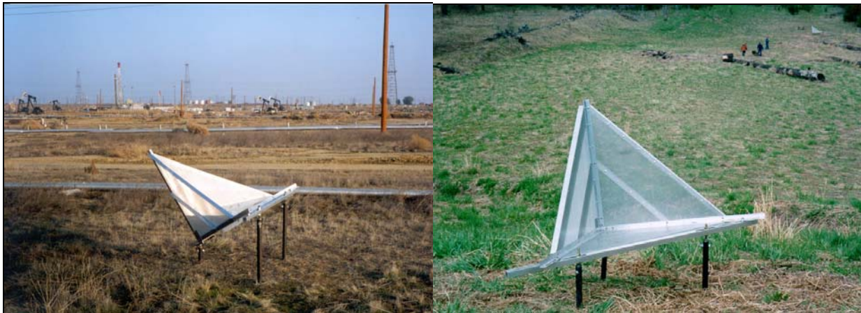
Figure 4. Photo. Reflectors can be used to mitigate the problem of temporal decorrelation.
