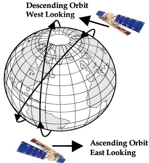
**Figure 6. Schematic. Polar orbiting satellites have an east looking and west looking perspective.<sup>(12)</sup>**
