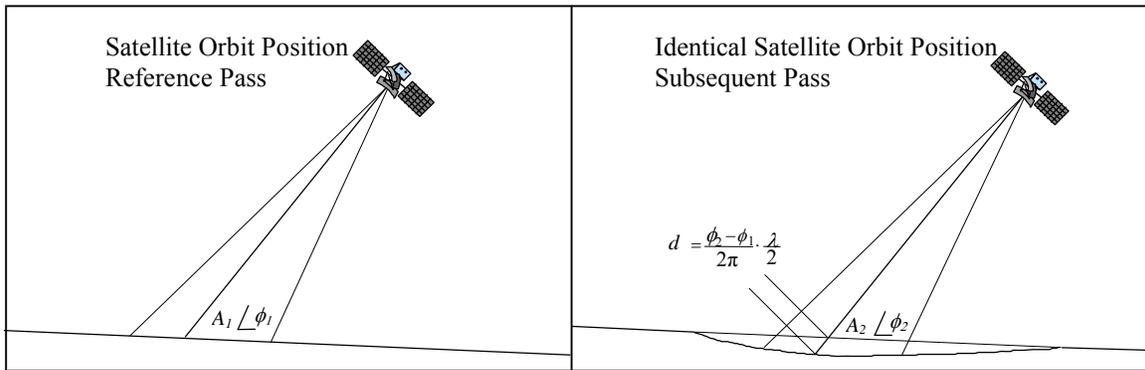
**Figure 2. Schematic. InSAR measurement of ground movement.**
