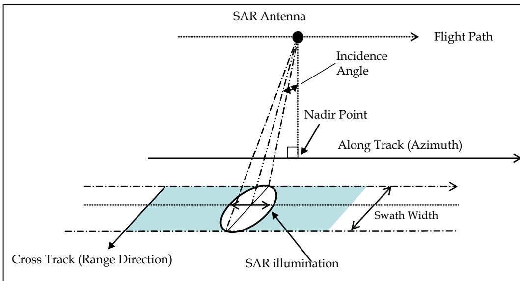
**Figure 1. Schematic. Geometry of synthetic aperture radar.**
