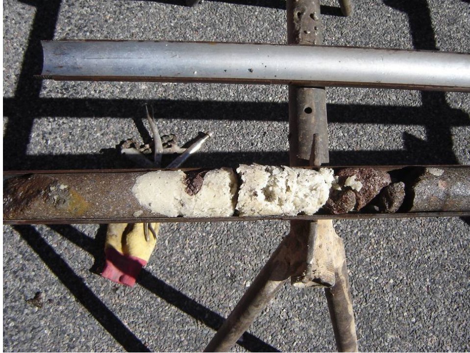
Figure 23. Photo. Light-colored, foamed PUR in core sample.
