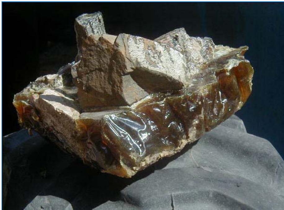
Figure 1. Photo. PUR and rock fragments test sample prepared at project site.
