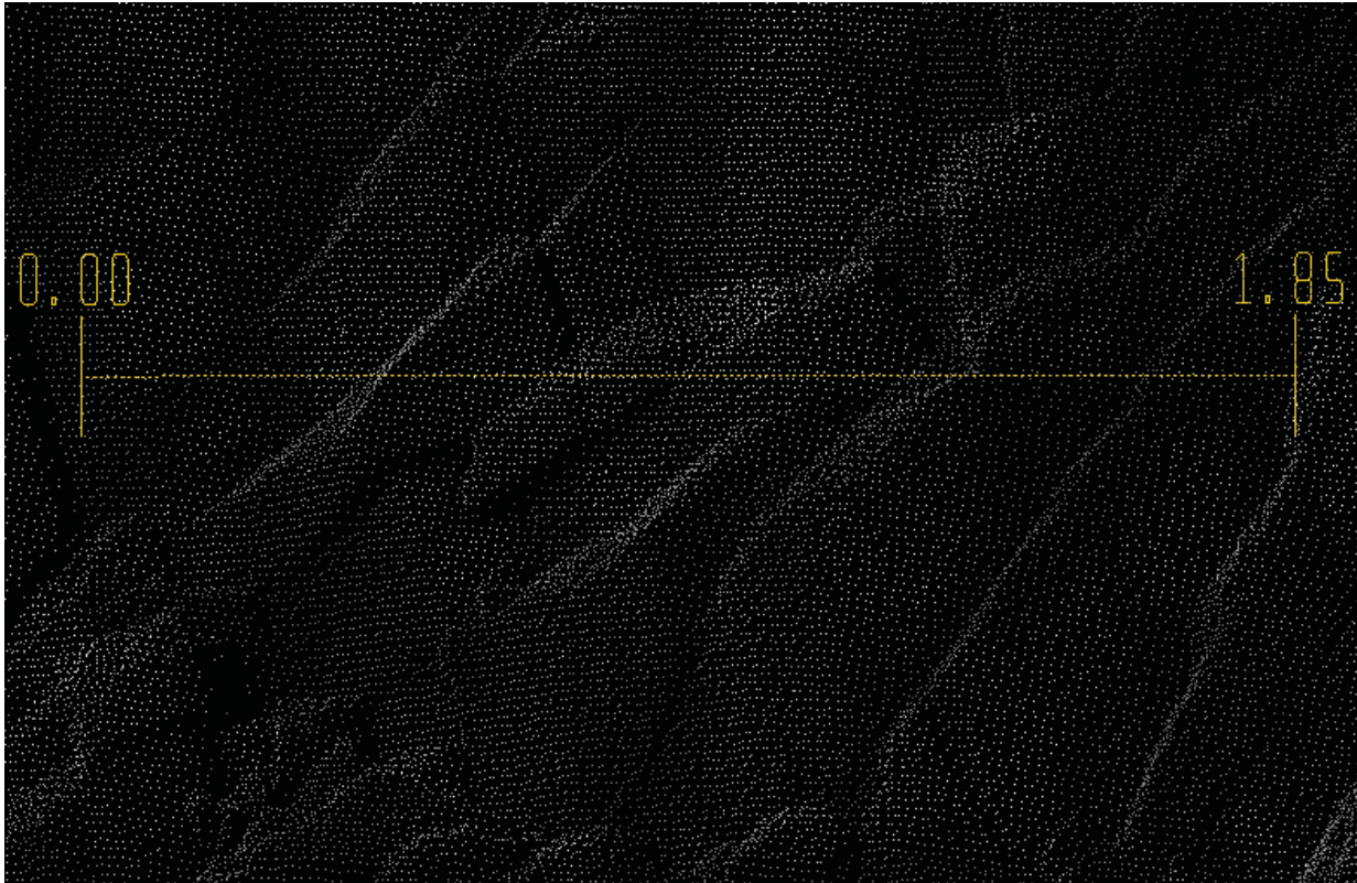
Figure 25. Schematic. Point cloud example. Ideal point cloud with a point spacing of about 1.5 cm (yellow ruler showing 1.85 meters).
