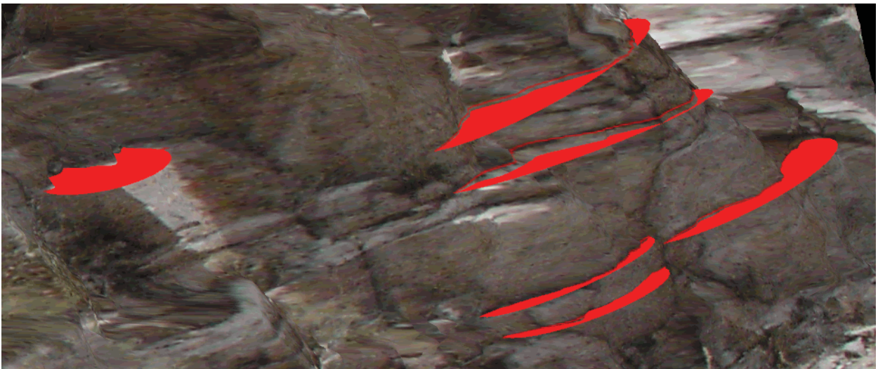
Figure 6d. Photo. Step 4 in photo draping procedure, three dimensional fracture orientations extracted from the traces.
