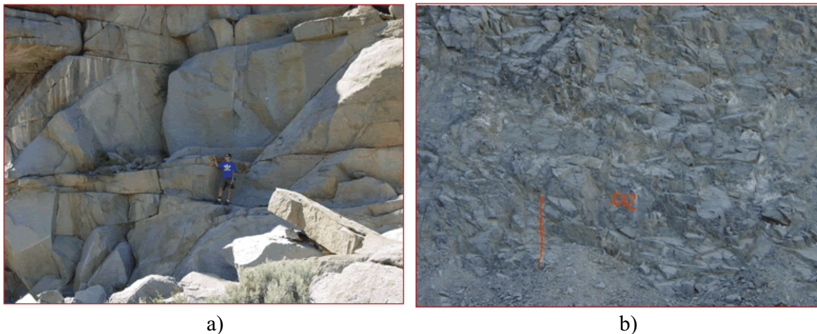
Figure 12. Photos. a) digital image with the proper density of fracture information, b) figure cannot be analyzed at its current scale (close-up image needed to provide appropriate level of detail).
