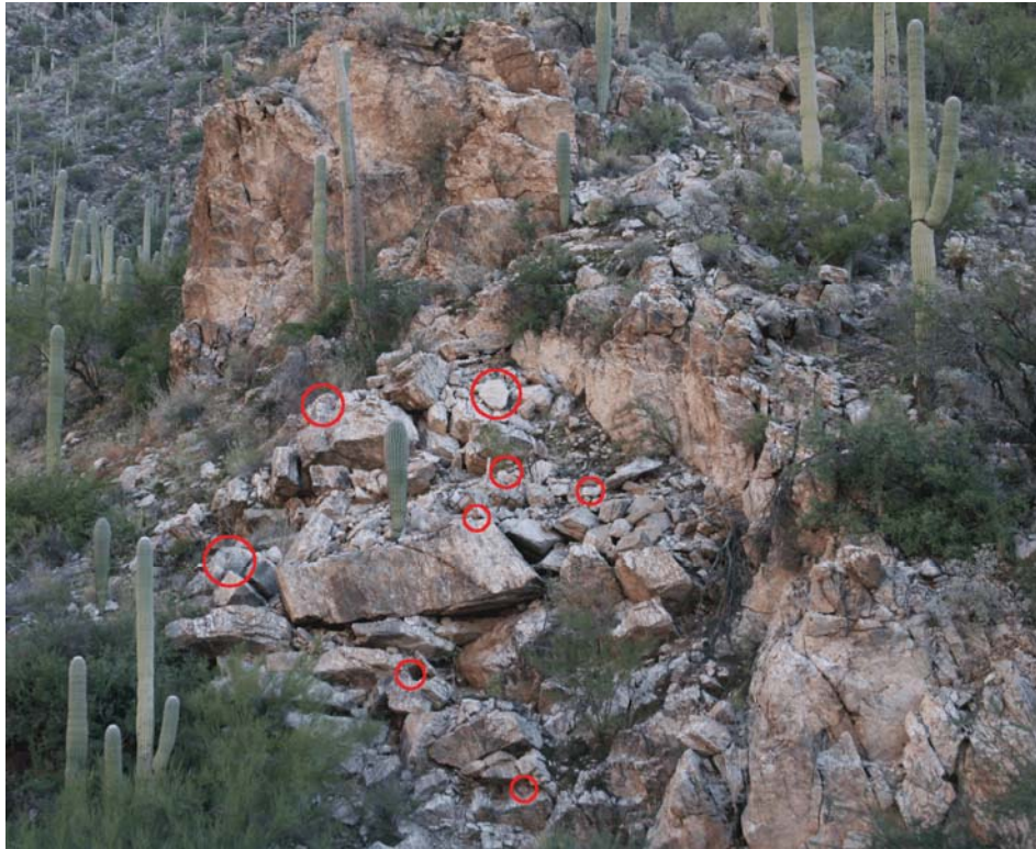
Figure 20a. Photo. Field site for testing change detection algorithms. Boulders marked with red circles were moved.
