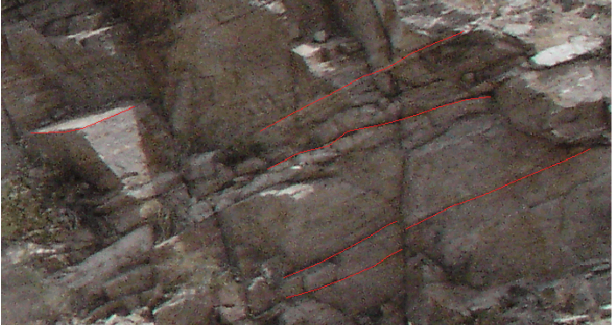
Figure 6c. Photo. Step 3 in photo draping procedure, delineate fracture traces on the digital image.
