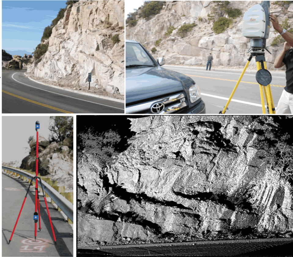
Figure 3. Photo. Scanning with the Leica ScanStation at Milepost 15 on Mt. Lemmon Highway. Point cloud shown in the lower right photo.
