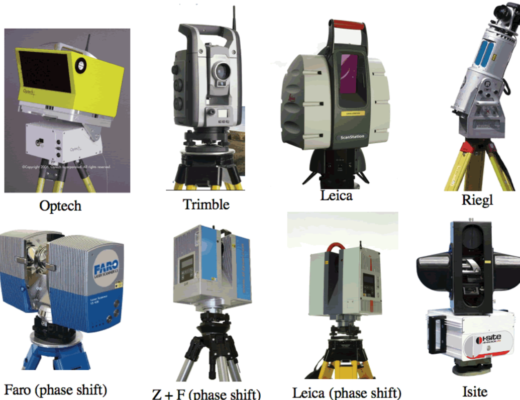
Figure 2. Photo. Examples of ground-based LiDAR scanners (time-of-flight unless noted otherwise, photos from 2006 models).
