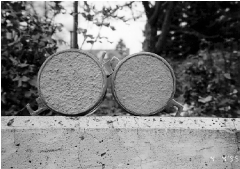
Figure E.2 Alderwood/Everett Dessication. Shown above are Alderwood loamy sand (left) and Everett loamy sand (right) after drying in an oven for 24 hours. Alderwood showed no separation from the cell walls, but dessication cracks were observable from the soil surface. Everett showed minimal to no crack formation.
