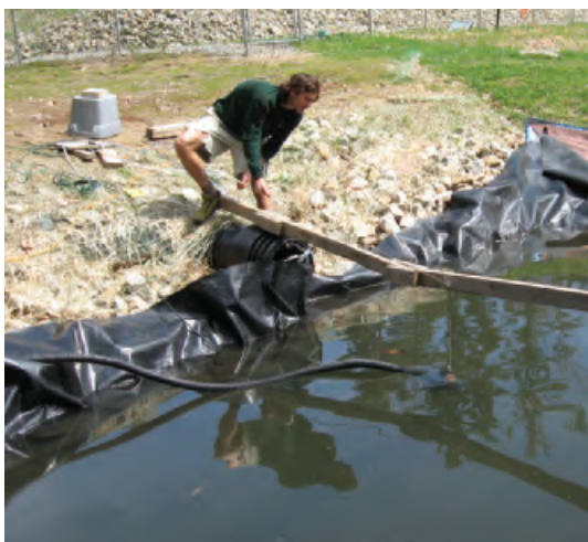
Graduate Student George Fowler begins the process of reducing sediments captured during a storm down to its actual mass.
