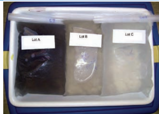
First flush samples taken from a storm after sealcoating. The sample on the left was taken from a parking lot recently sealcoated while the sample to the right was taken from an unsealed reference lot during the same event.
