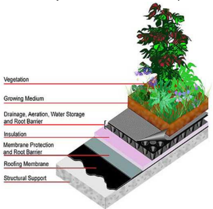
Figure 1: Structure of a Green Roof (Source: heatusa.com)
