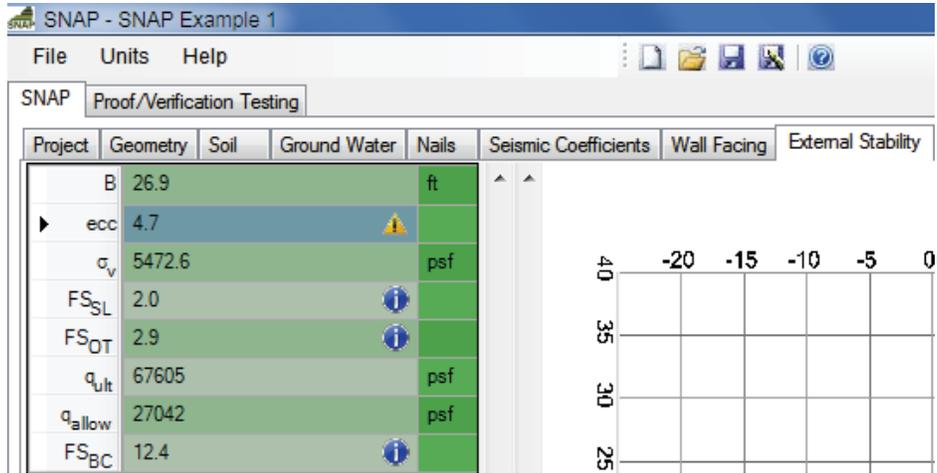
**Figure 66. Screen Shot. Example 1, External Stability analysis results.**
