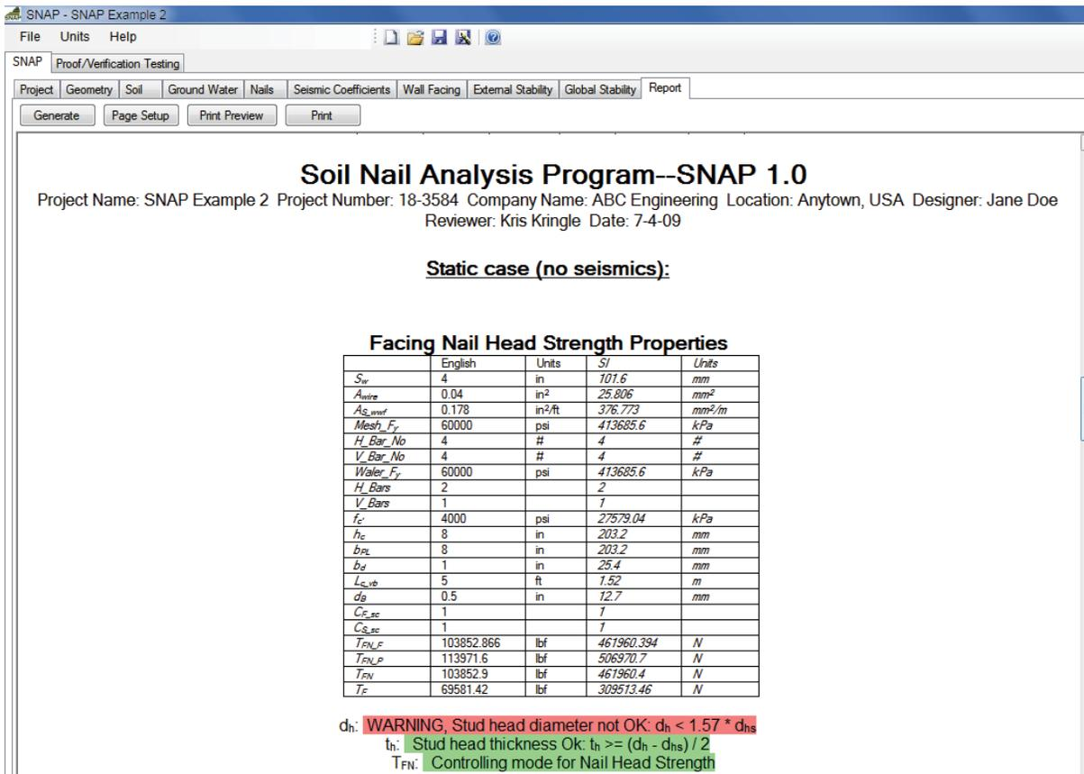
Note:  $D_H$  is stud diameter and  $D_{HS}$  is stud body (reversed from document FHWA-SA-96-069R)
