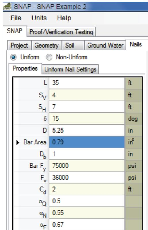
**Figure 73. Screen Shot. Example 2, the Nail Properties tab.**
