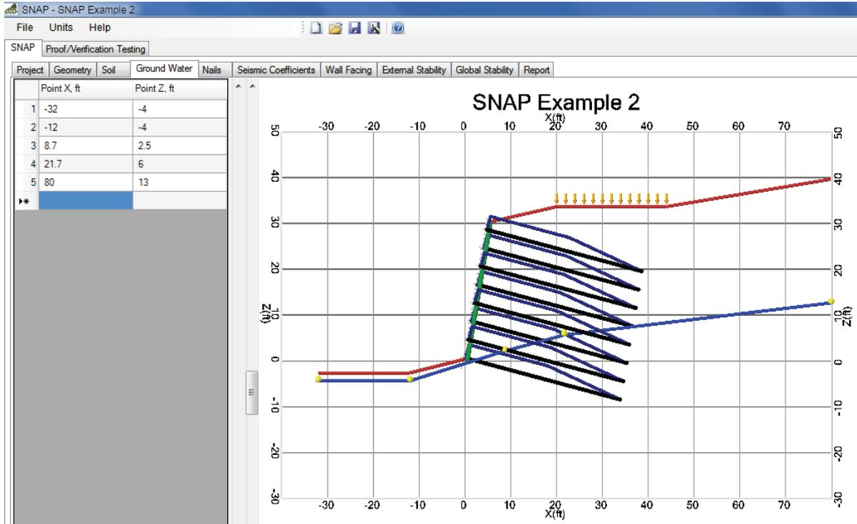
**Figure 72. Screen Shot. Example 2, the Groundwater tab.**
