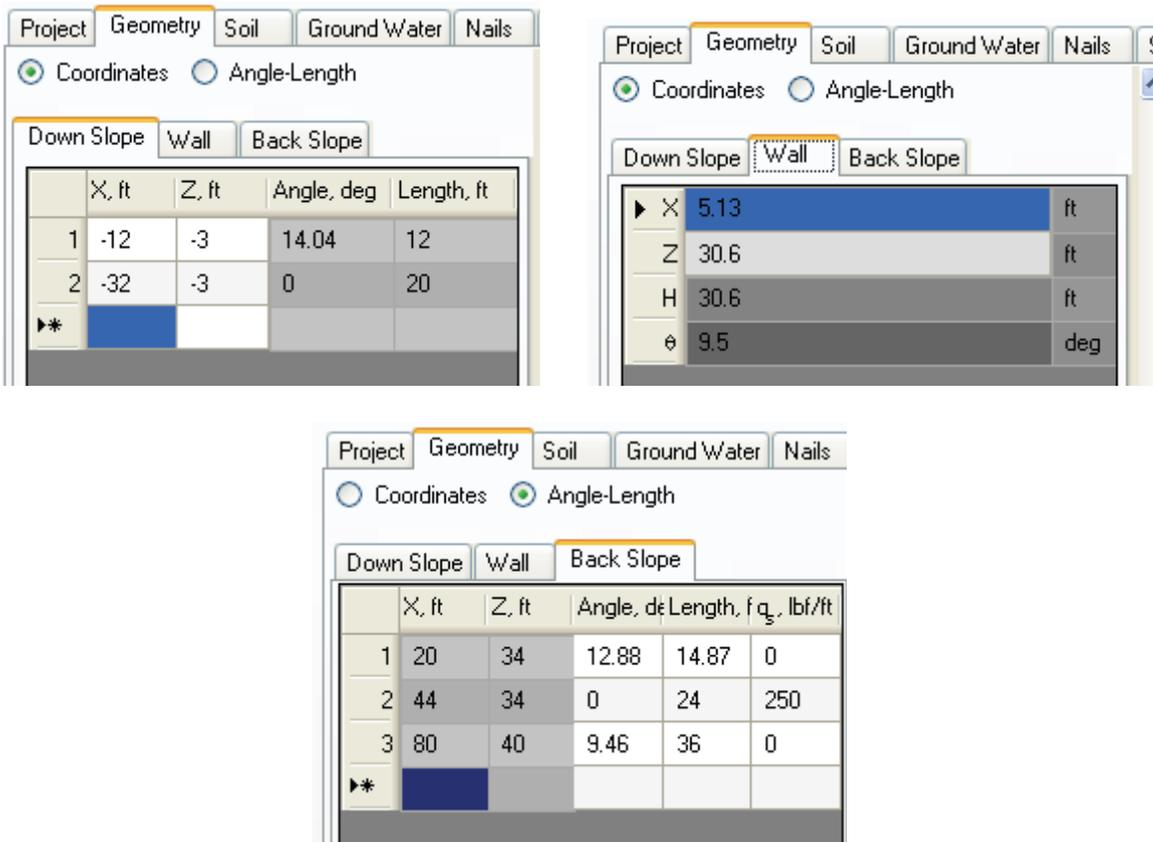
**Figure 69. Screen Shot. Example 2, the Geometry tab.**
