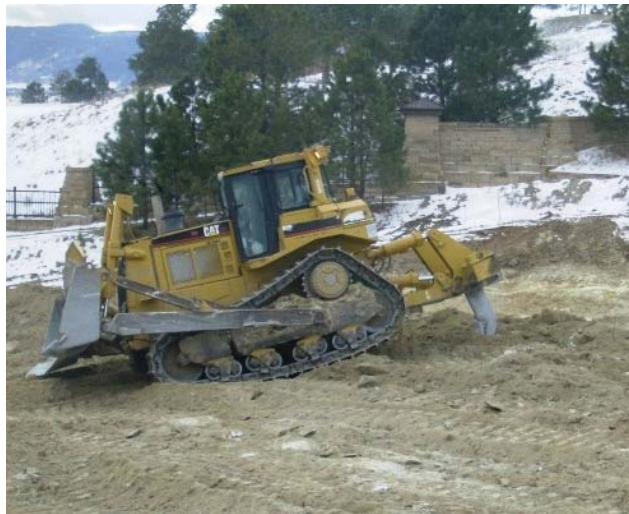
Figure 21. Photo. Bulldozer with an integral ripping attachment.
