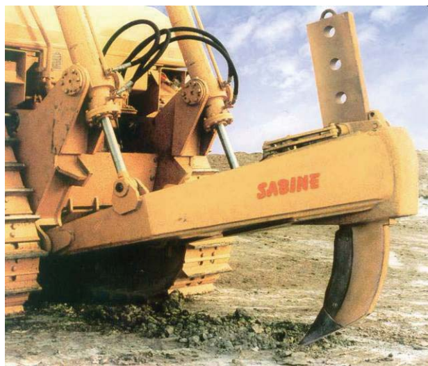
Figure 22. Photo. Typical hinge- or radial-style ripper (Nichols and Day 2005).
