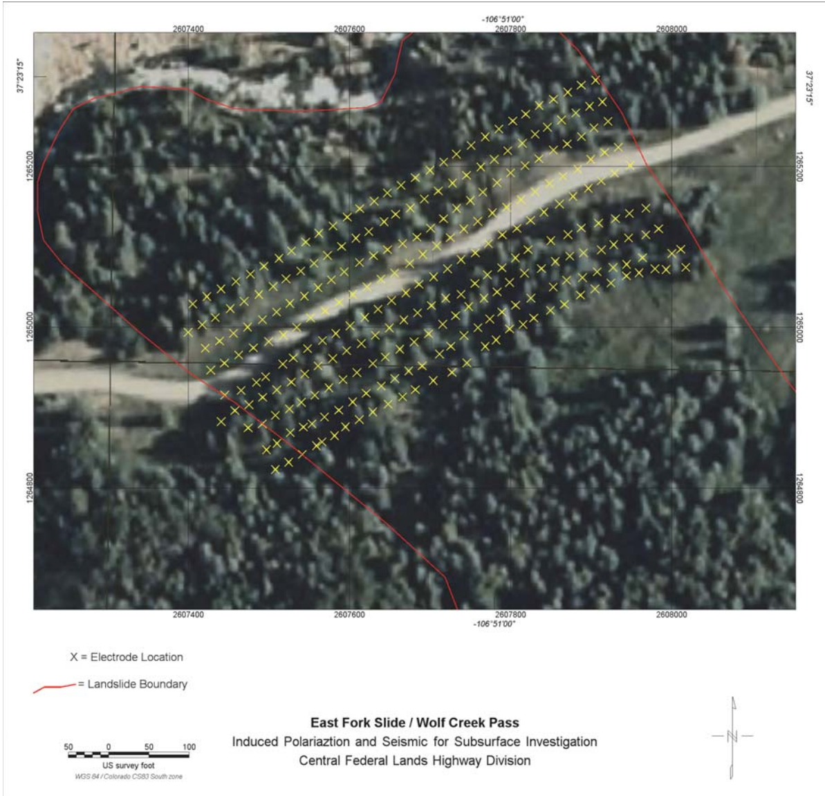
Figure B2. Image. Yellow X's are the receiver (geophone) locations for the East Fork survey.
