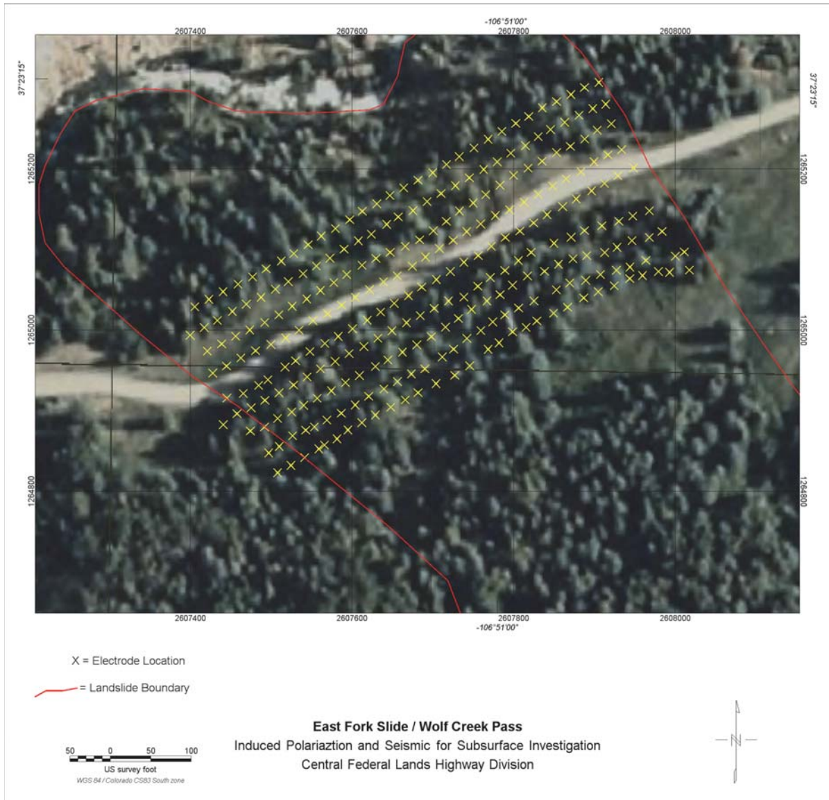
Figure A2. Map. Yellow X's are the receiver (electrode) locations for the East Fork survey.
