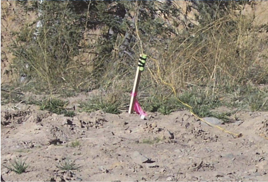
Figure 13. Photo. Poulter charge on short pole.
