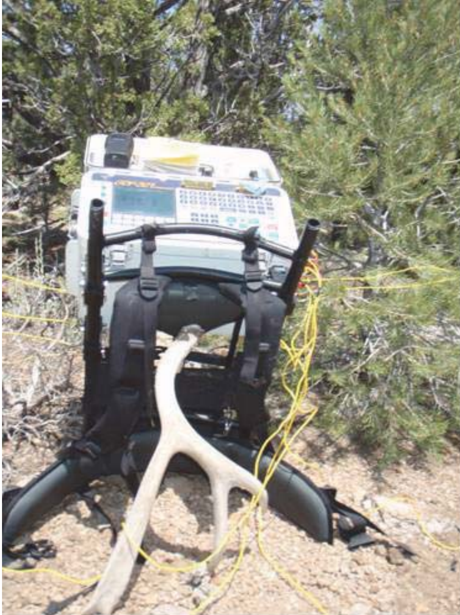
Figure 6. Photo. Zonge GDP-32 receiver configured for IP on backpack.
