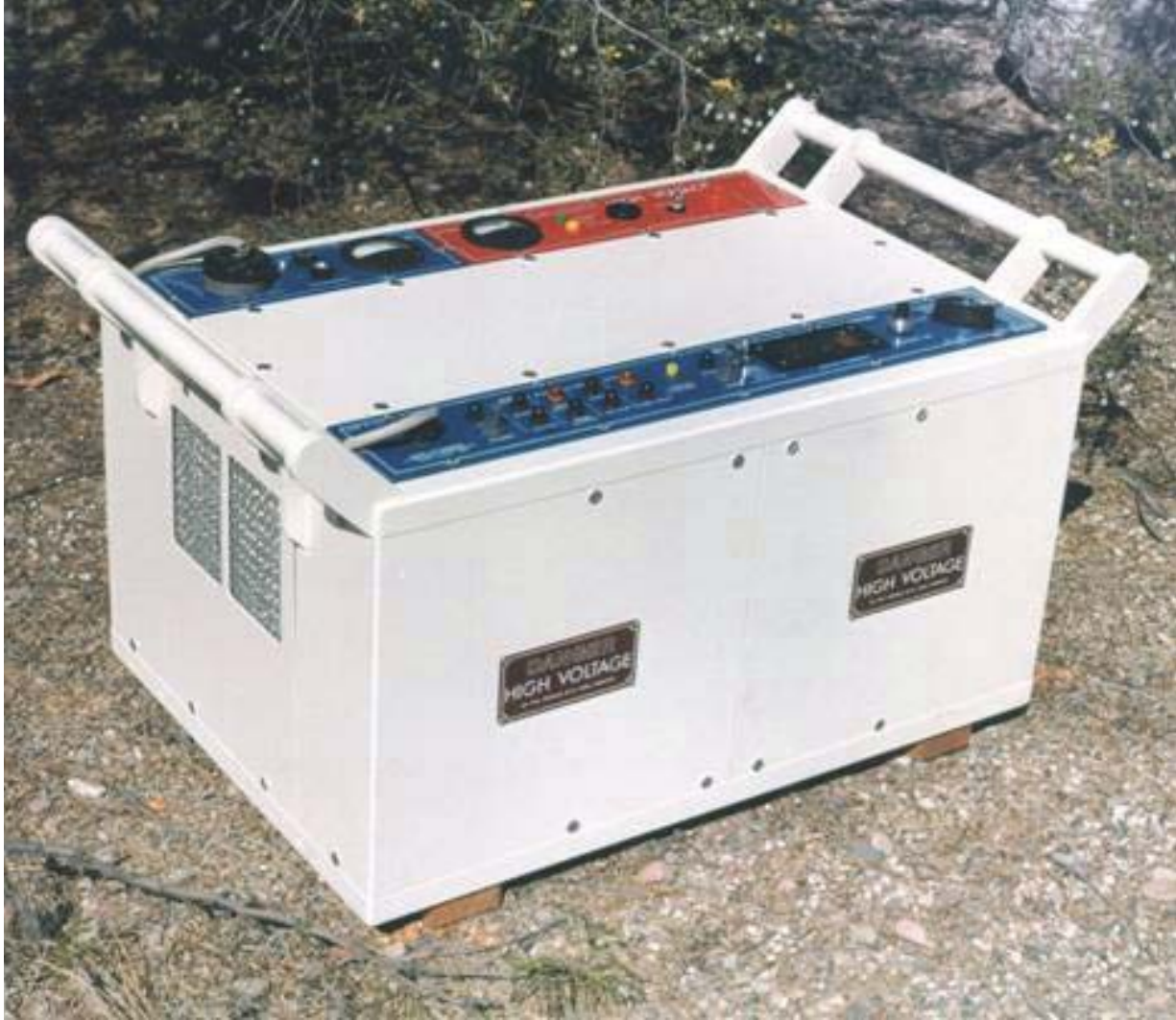
Figure 4. Photo. Zonge IP Transmitter.
