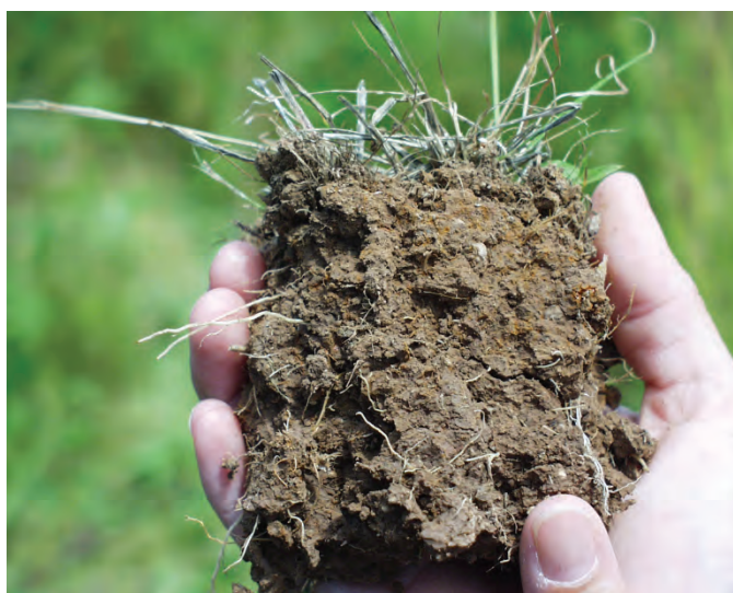
Figure 27. In this example, the layer of redox concentrations begins at the soil surface and is slightly more than 2 in. (5-cm) thick.
