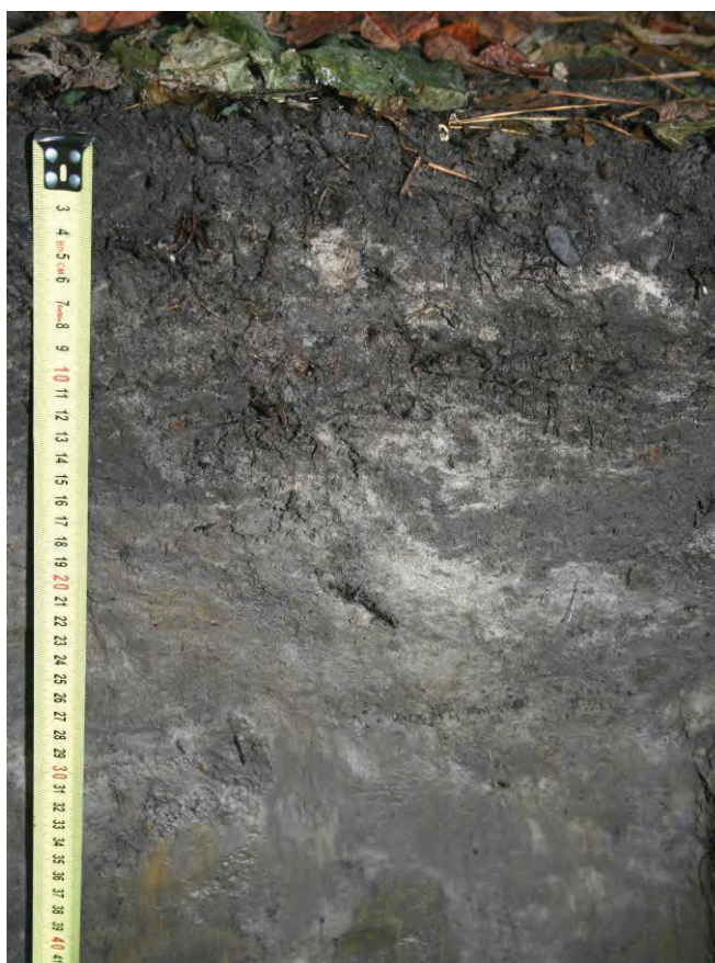
Figure 26. Redox depletions (lighter colored areas) are scattered within the darker matrix. Scale is in centimeters.
