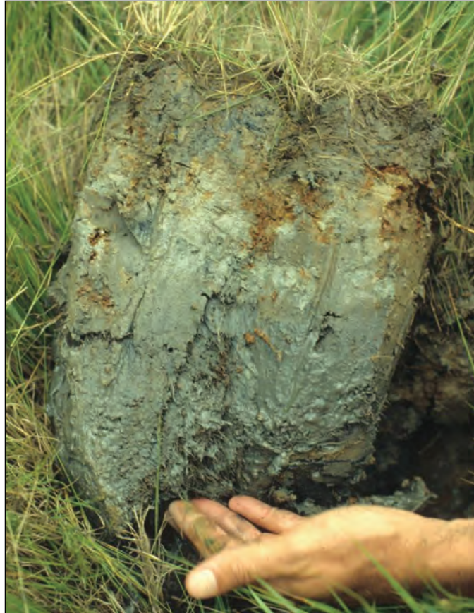
Figure 22. This soil has a gleyed matrix in the lowest layer, starting about 7 in. (18 cm) from the soil surface. The layer above the gleyed matrix has a depleted matrix.
