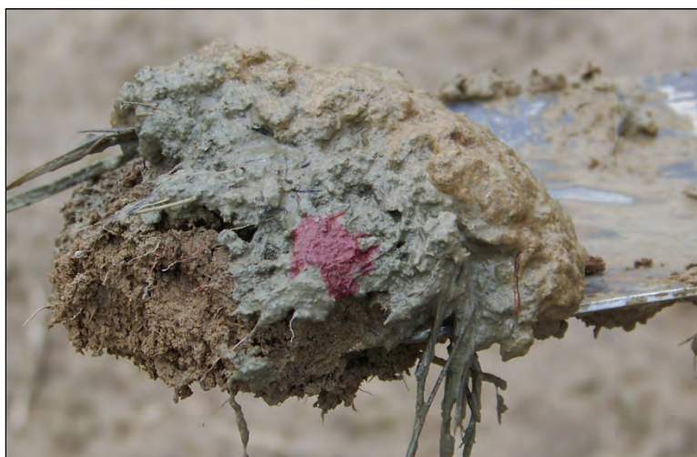
Figure 57. When alpha, alpha-dipyridyl is applied to a soil containing reduced iron, a positive reaction is indicated by a pink or red coloration to the treated area.
