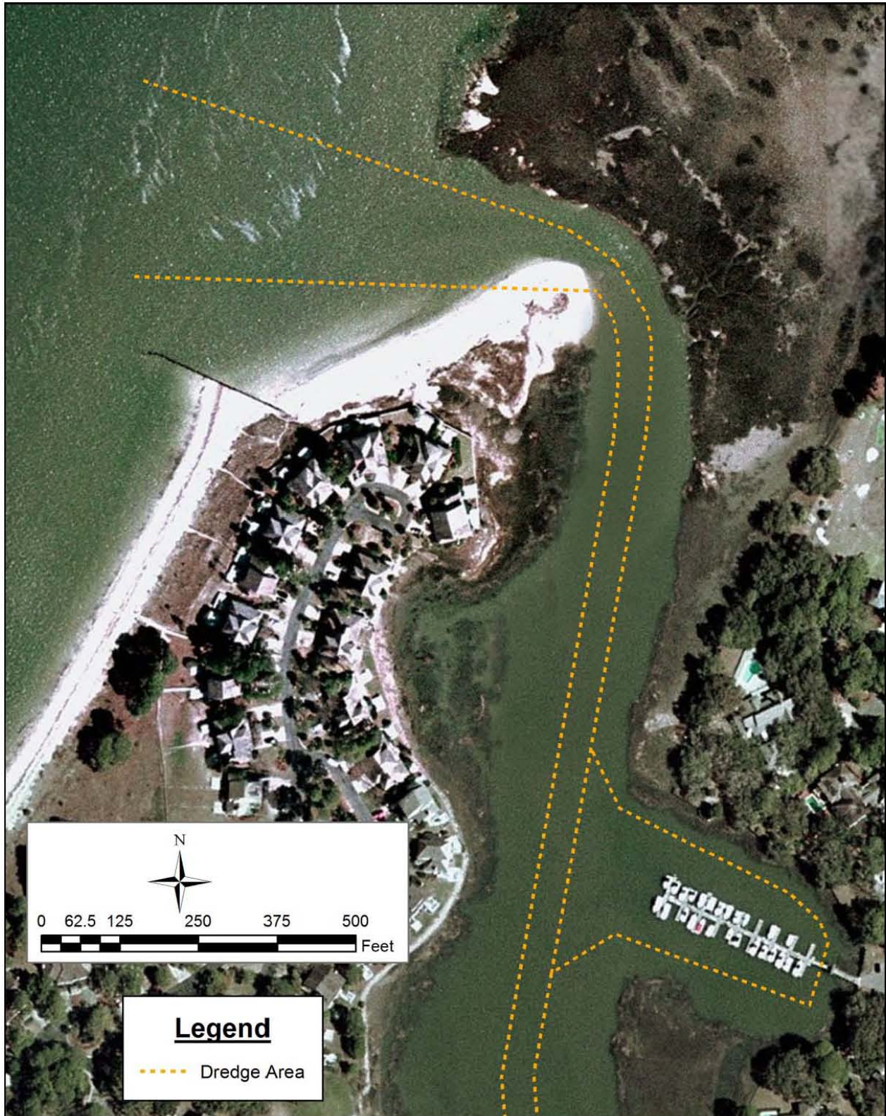
Figure 1-4: Braddock Cove Creek Mouth and Gull Point Marina Areas to be Dredged
