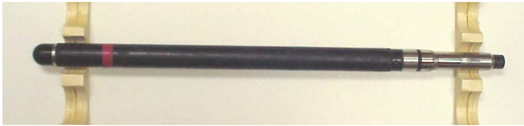
Figure 3. Mount Sopris 2PGA-1000 Poly-Gamma probe
