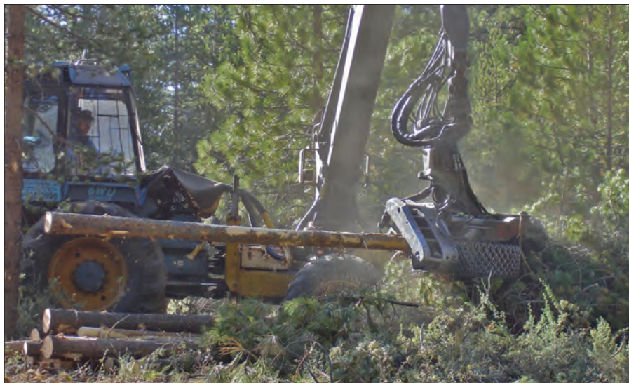
A worker operates a cut-to-length harvester during a forest-thinning project.
