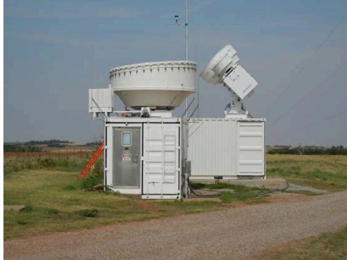
Figure 1. KAZR installation at SGP (foreground) with SACR (background).
