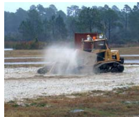
The All-Purpose Remote Transport System (ARTS) perform range clearance functions with its flail attachment
