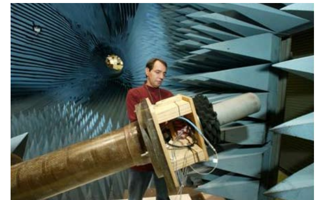
Radio Frequency Tapered Anechoic Chamber
