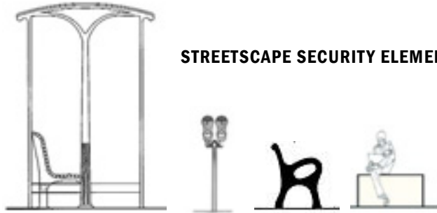
Hardened Street Furniture
