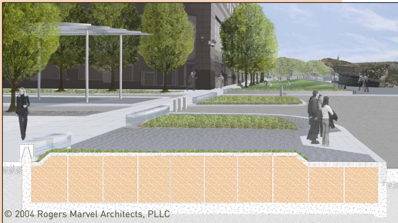
The Tiger Trap™ system can protect against a vehicle attack without impeding open public spaces.
