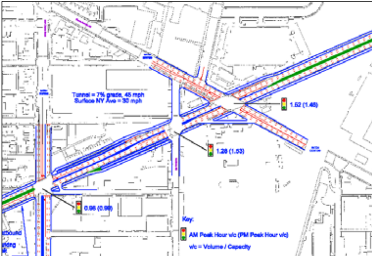
Preliminary concept plan for Tunnel Alternative as shown in DDOT's New York Avenue Corridor Study.
