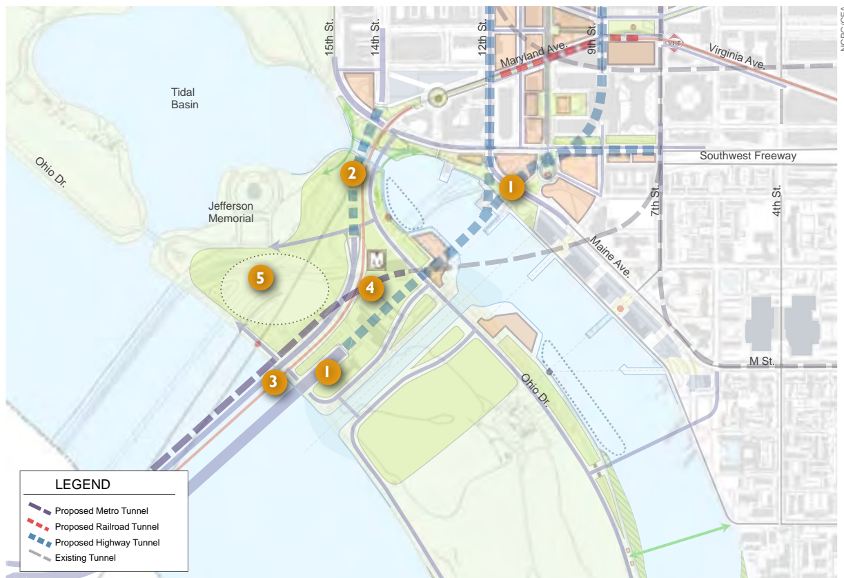
Proposed tunnels that will allow creation of the Jefferson Memorial Festival Green and connect Potomac Park to the National Mall.
