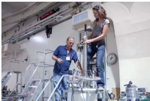
NCNR's Bill Clow and Elisabeth Carpenter place a sample into a top-loading ^3\text{He} cryostat
