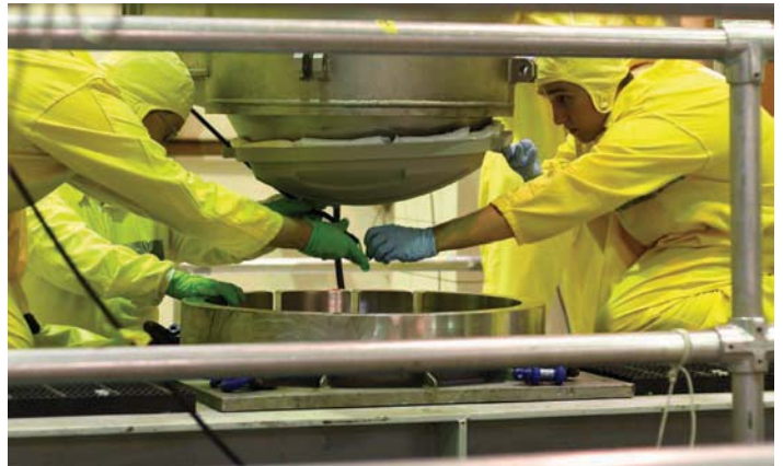
FIGURE 2: Cask is aligned in a spent fuel transfer operation.
