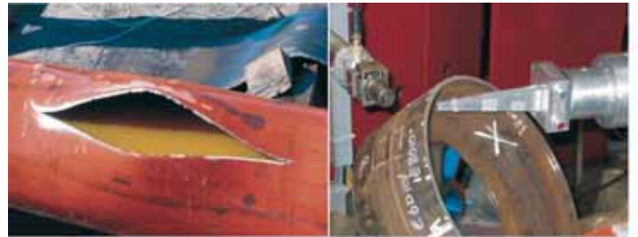
FIGURE 1: Left: Circumferential rupture in the hydrotest, and Right: measurement geometry for the corresponding hoop direction.
