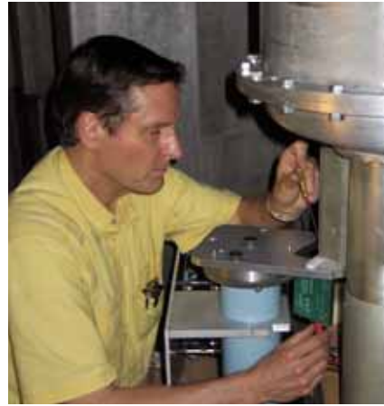
FIGURE 6: Jeff Ziegler installs one of his Preamplifier-Amplifier-Discriminator modules in the High Flux Backscattering Spectrometer.
