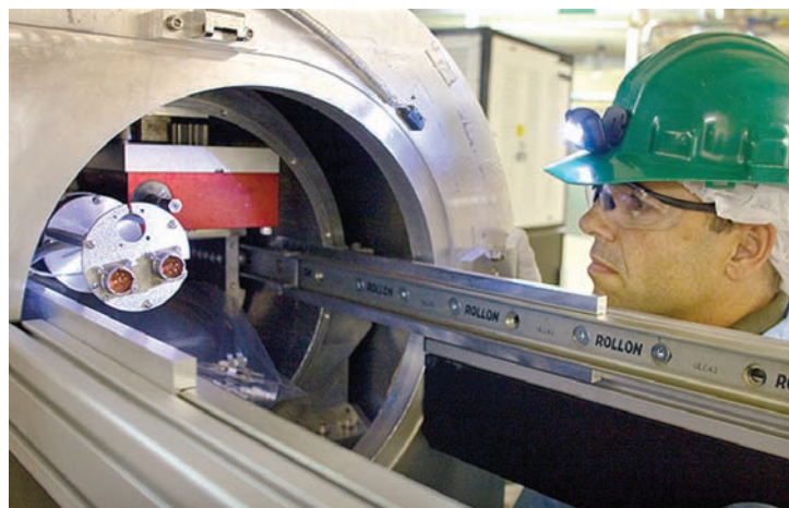
More than 30 diagnostic instruments have been installed at NIF, such as the gamma reaction history device (left) and the gated x-ray imager (above).
