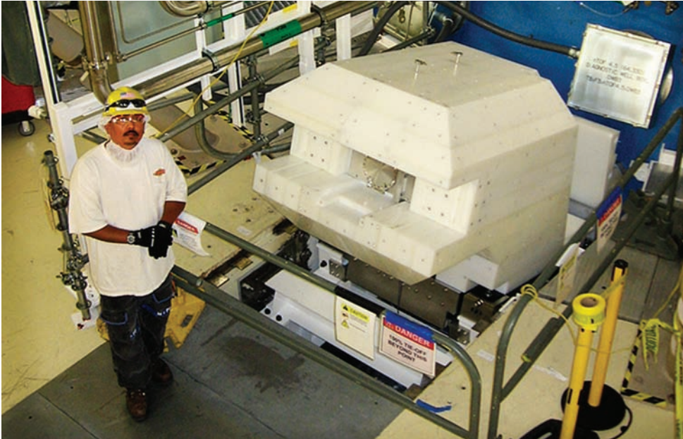
The magnetic recoil spectrometer provides a novel approach to measuring neutron time of flight by converting neutrons to protons, which have a higher interaction probability within the detector.
