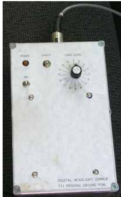
Figure 14. Photo. Headlamp controller box.
