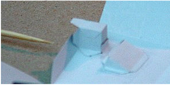
The inside of the spacecraft's back panel: left is PFS sub-assembly fitted in the cut-out (C1), right the star tracker platform mounted in the cut-out (C2)
