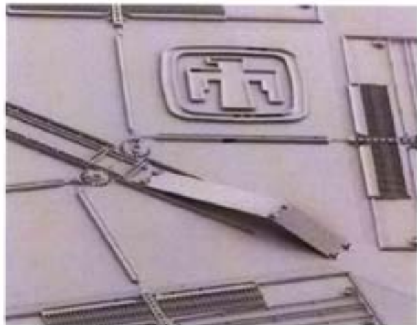
Image 11. Hinged Polysilicon Mirror and Drive Motors. (Photo Courtesy of Sandia National Laboratories, SUMMIT™ Technologies.)
