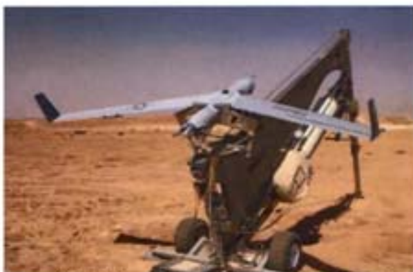
Image 05. A Scan Eagle UAV sits on its catapult prior to launch in Al Asad, Iraq. (Photo Courtesy of the U.S. Marine Corps/Gunnery Sgt. Shannon Arledge.)
