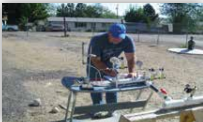
Chris Orme from INL performs feasibility testing on the use of a membrane based gas dehydration process in Marsing, Idaho.
