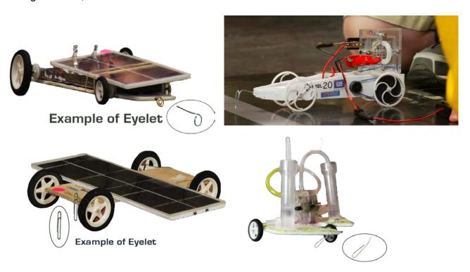
9. The solar vehicle must be structurally sound without the solar panel. The solar panel cannot be used as the chassis (body of the car). Teams are **NOT** allowed to bolt the axles and wheels to the solar panel—the car must be three dimensional.
