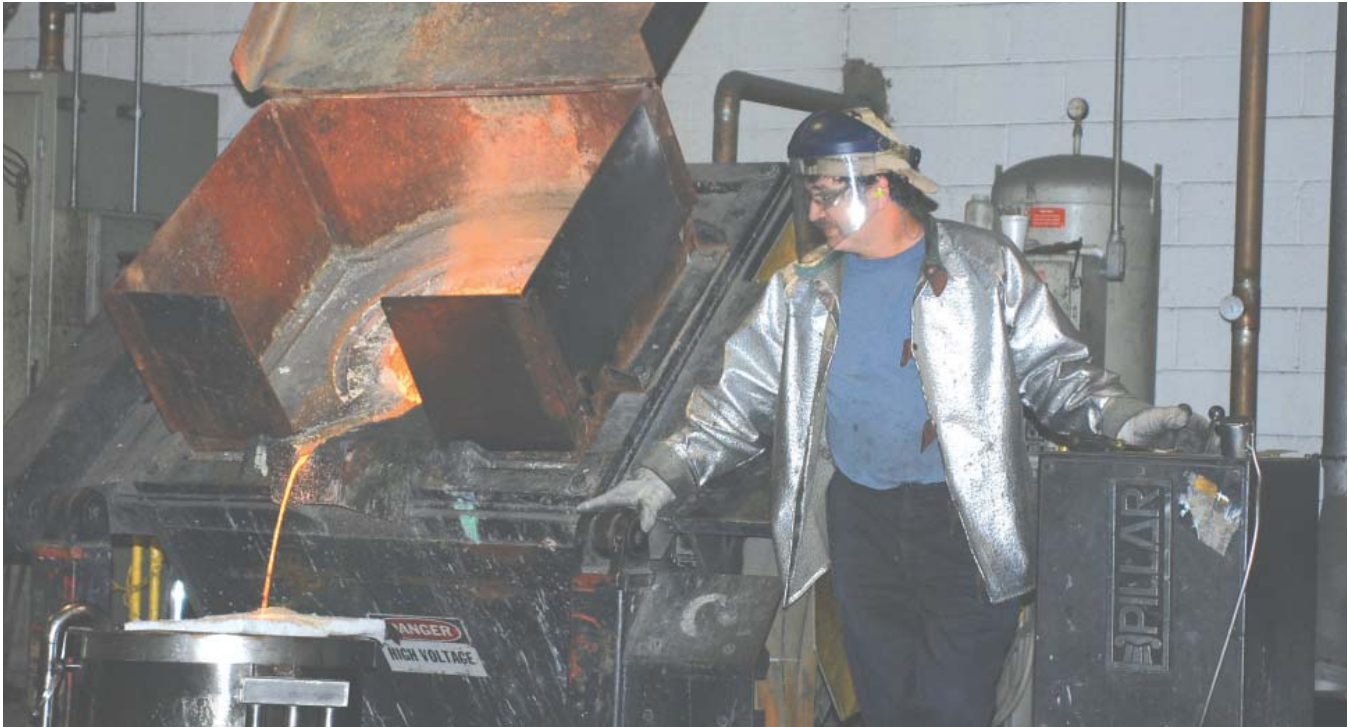
OPM smelter operator processes recycled metals and pours them into selected molds for cooling.
