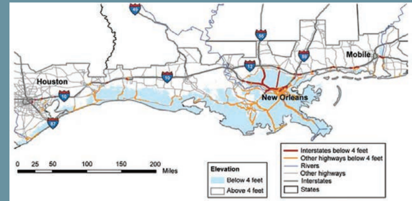
Figure 12: The Gulf coast area roads at risk from four feet of long-term relative sea level rise. Source: U.S. Global Change Research Program, 2009
