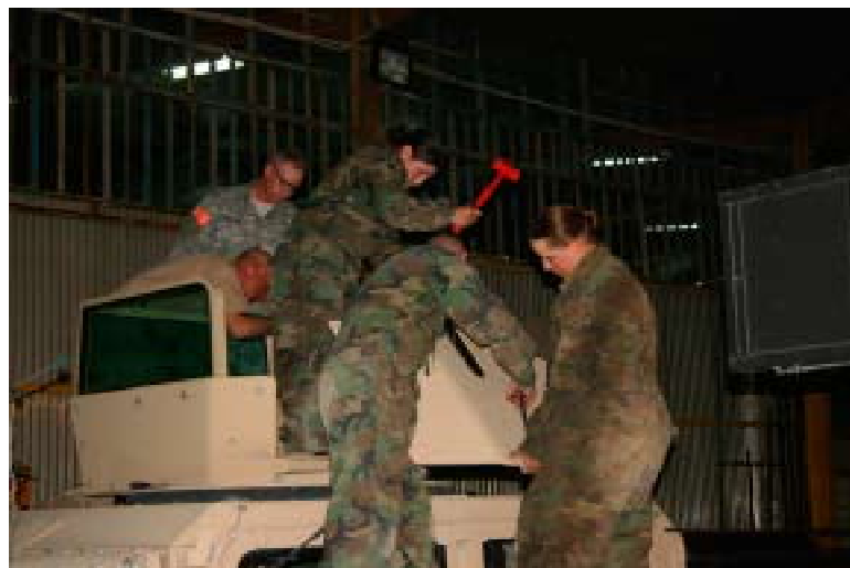
photo courtesy of 610th BSB Soldiers of Company B, 610th Brigade Support Battalion, work on gun turrets for humvees. The Soldiers added plexiglass and other improvements to the vehicles.
