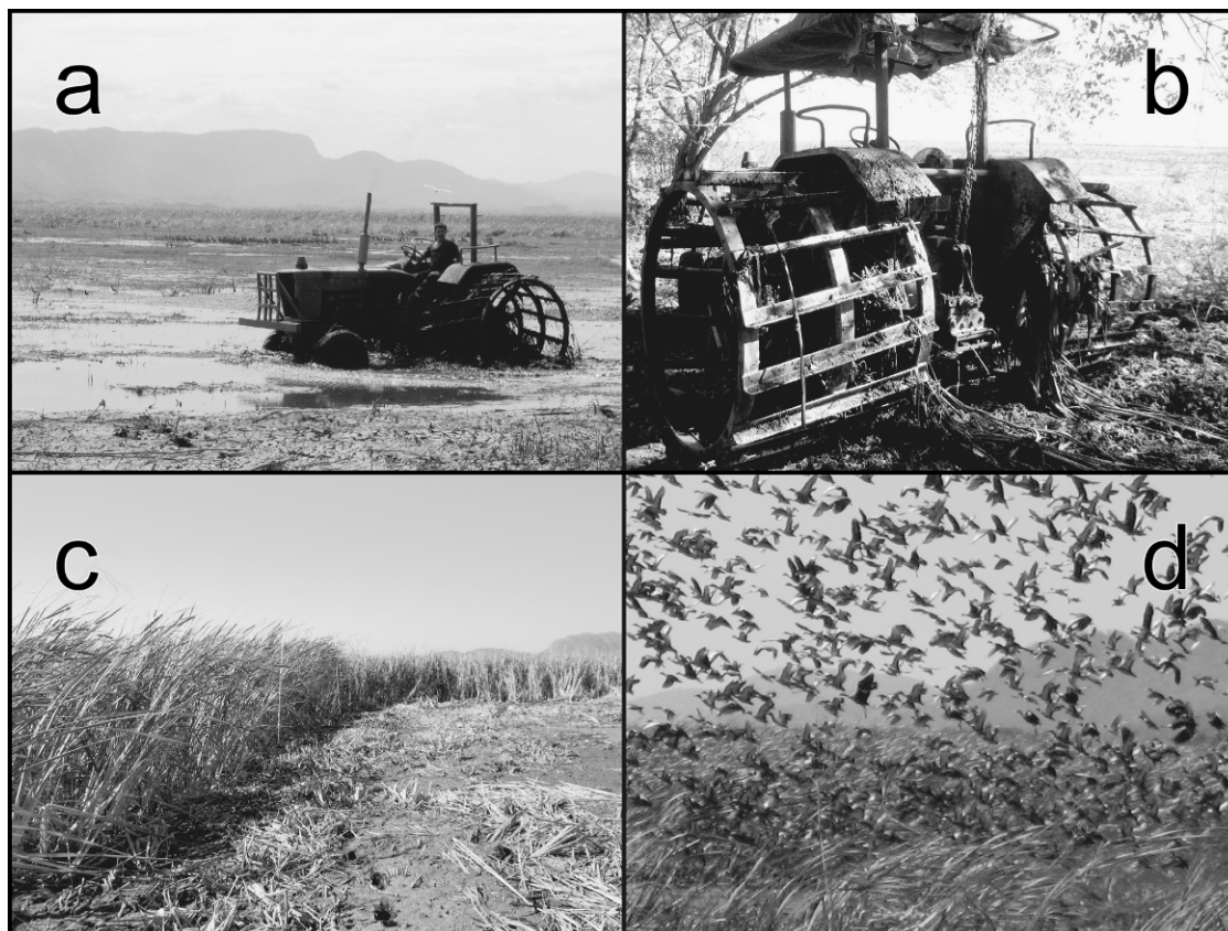
FIG. 1. Photos from Palo Verde Marsh, Palo Verde National Park, Costa Rica, depicting: (a, b) a tractor with metal paddle wheels used to remove Typha via a mechanical disturbance that is called fanguero; (c) the edge of a plot where Typha was removed via fanguero, and (d) migratory birds utilizing and flying away from a plot where Typha was removed via fanguero. Most of the individuals in the last photo are Black-bellied Whistling Ducks ( Dendrocygna autumnalis ), which were especially numerous after Typha removal (photo credits: M. J. Osland).
