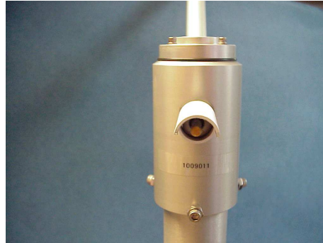
Figure 14. Temperature sensor should protrude under solar radiation shield.
