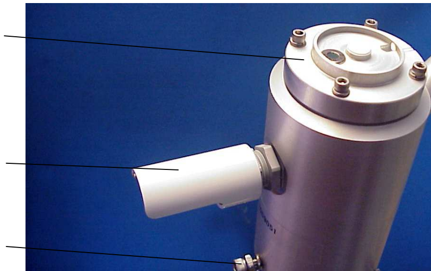
Figure 13. Ensure the ambient temperature sensor probe is extended, the white shield is positioned as shown, and top plate and solar/IR sensors are both level.
