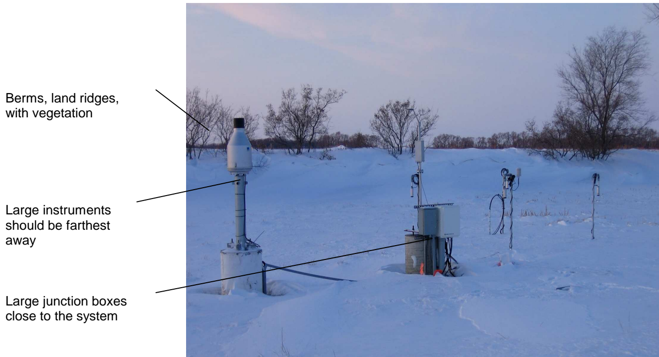
Figure 9. Subtle site issues that can create unwanted local wind turbulence.
