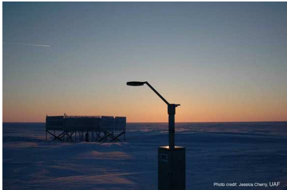
Figure 2. TPC at the US Department of Energy's North Slope Alaska site. A Double Fenced Intercomparison Rain gauge is located in the background.
