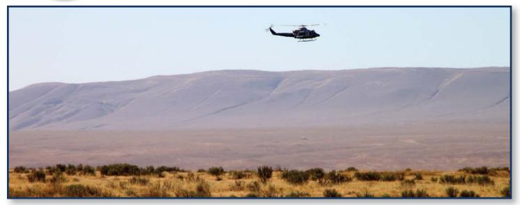
Officials at the Hanford Site in Washington State are using an innovative, cost-saving approach to measure radioactive contamination in the soil. In late September, a Bell 412/HP helicopter made several passes over a portion of the 586-squaremile government site that produced plutonium from the 1940s to the 1980s. Detectors and electronics on the aircraft recorded the type and location of contamination.
