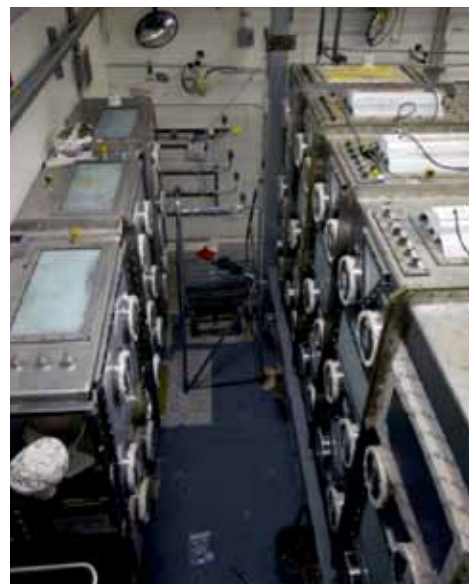
(above) A narrow space between the glove boxes in Room 230C (HC-230C-4 at left, HC-230C-3 at right) complicated their removal.
